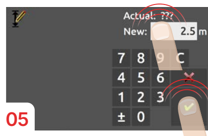
05 Enter "2.5m" as the height (the height between your bucket and the bottom of the trench) then confirm.
